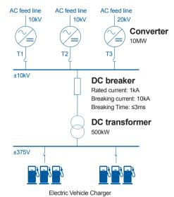
When fault occurs at MVDC circuits, DC circuit breaker will isolate the fault and healthy parts operate continuously. Meahwhile, operational experiences of DC circuit breaker are accumulating.
